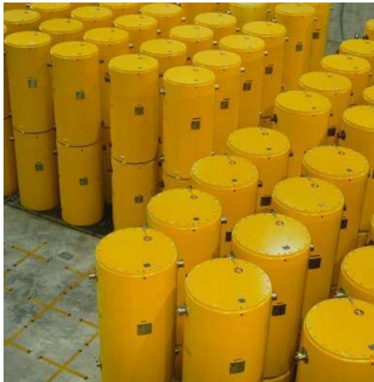
Figure D–2: CASTOR-THTR containers in the Ahaus interim storage facility (Copyright: GNS)
