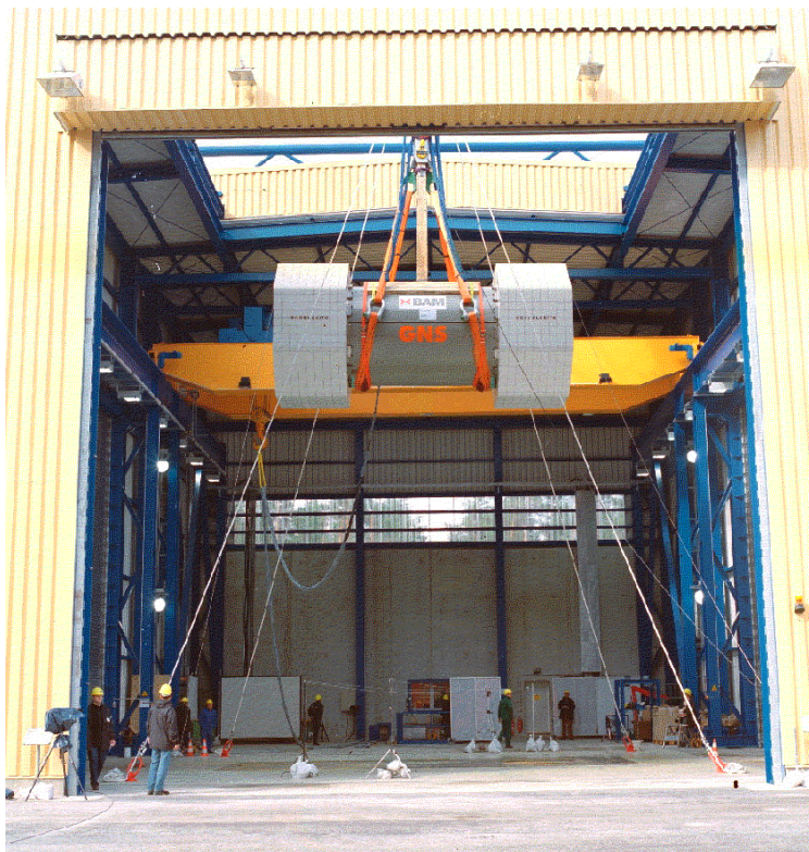
Figure G-2: Drop test of a spent fuel assembly transport and storage container at the new Federal Institute for Materials Research and Testing (BAM) test facility in 2004 (copyright: BAM).
