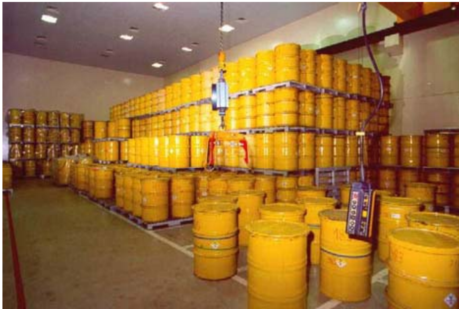
Figure H-1: Exit hall of the "Central radioactive waste treatment and disposal facility" (Zentralstelle zur Behandlung und Beseitigung radioaktiven Abfalls - ZRA) at the Hahn-Meitner Institute, with the interim storage volume as at September 2004. Being a State collecting facility of the Land Berlin, the ZRA accepts low- and medium-active waste arising from uses in industry and trade, medicine, and research and teaching. (Copyright: HMI)
