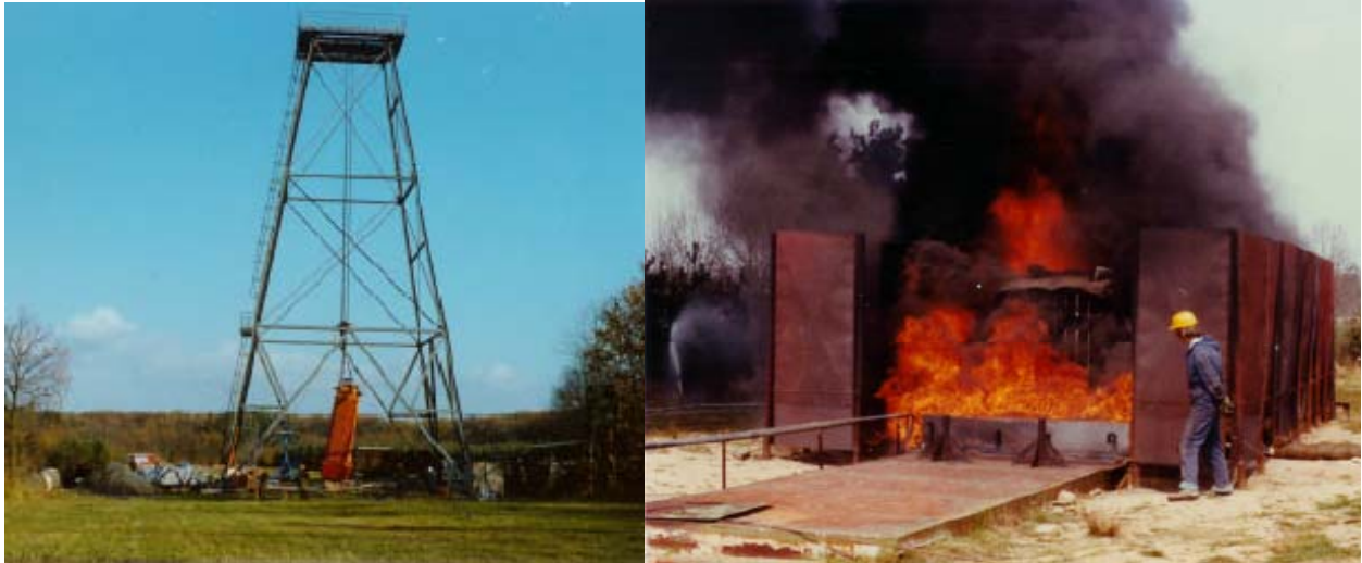
Figure G-1: First drop test and fire exposure test of a fuel assembly transport container for radioactive waste in original size from a height of 9 m at the test facility of Federal Institute for Materials Research and Testing (BAM) in Berlin in 1978 (copyright: BAM).
