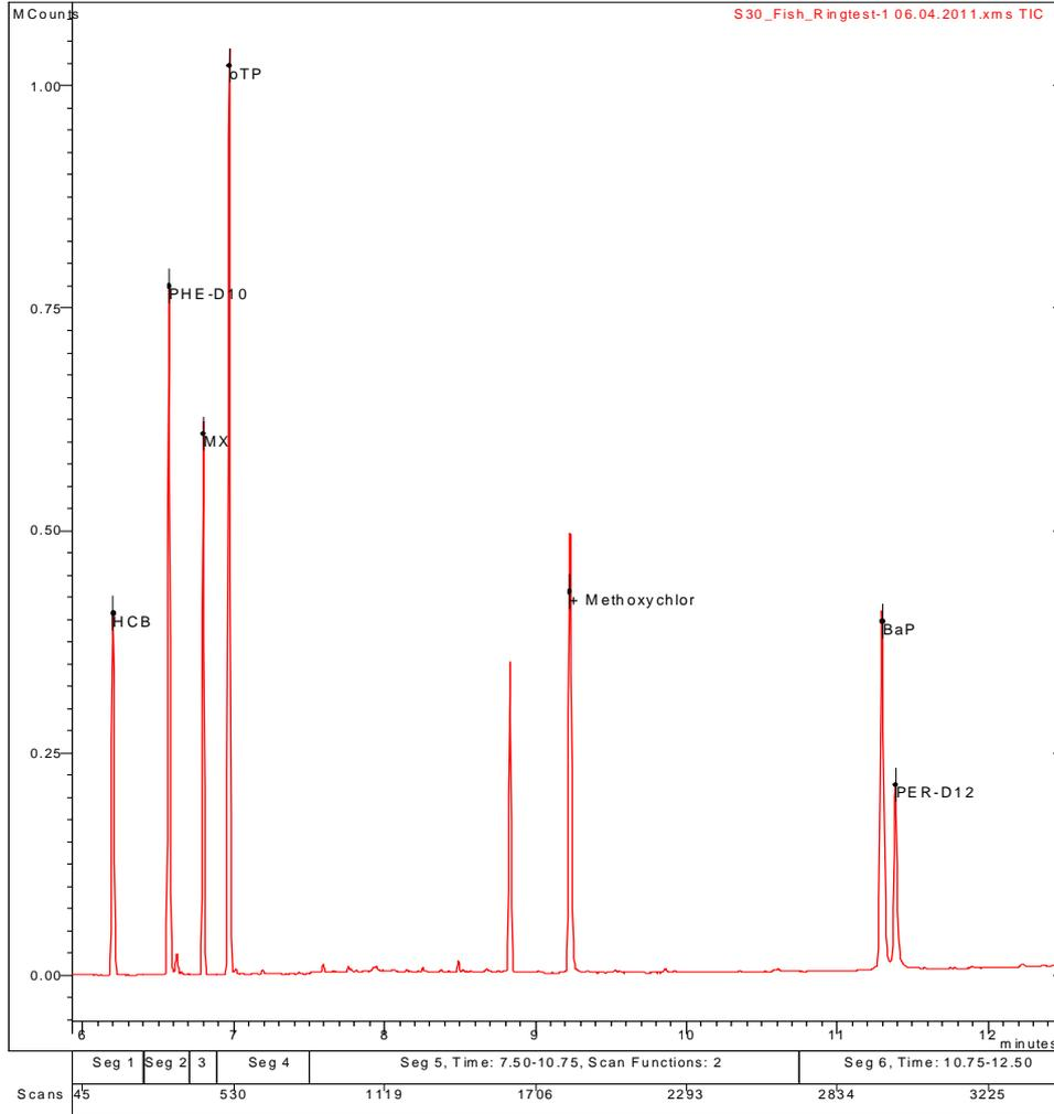
Figure 11: Chromatogram of a processed fish extract (uptake day 5)
