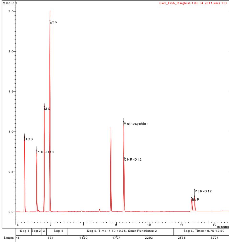
Figure 12: Chromatogram of a processed fish extract (deuration day 1)
