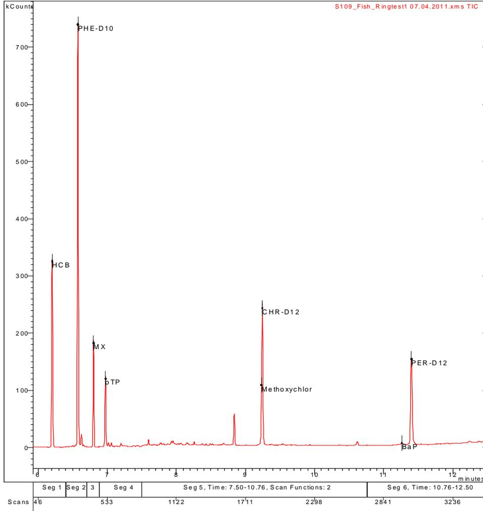
Figure 13: Chromatogram of a processed fish extract (depuration day 28)
