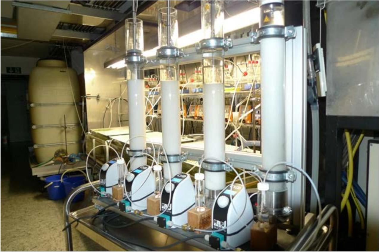
The water in the test vessels was aerated via a stainless steel capillary. Observations were made throughout the test period on fish behavior and mortality. Temperature, pH and the oxygen concentrations in the test vessels were measured daily. The light/dark cycle was adjusted to 12/12 hours and light intensities were measured once during the test.
