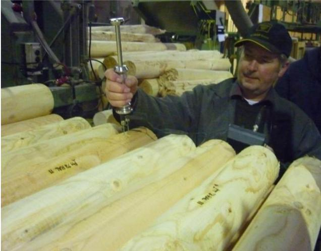
The electrical resistance measurement can be performed automatically. Wood moisture measurement is performed and controlled by an employee. Measurement is supported by computer and the measured values can be digitally recorded and documented.
